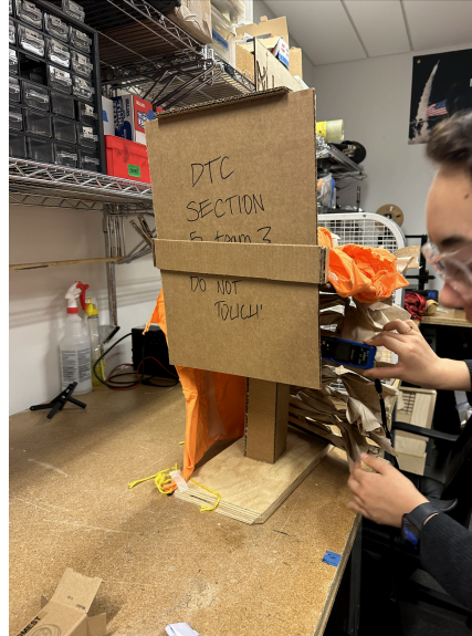
Fig. D4. Measuring wind speed behind the straw mockup
