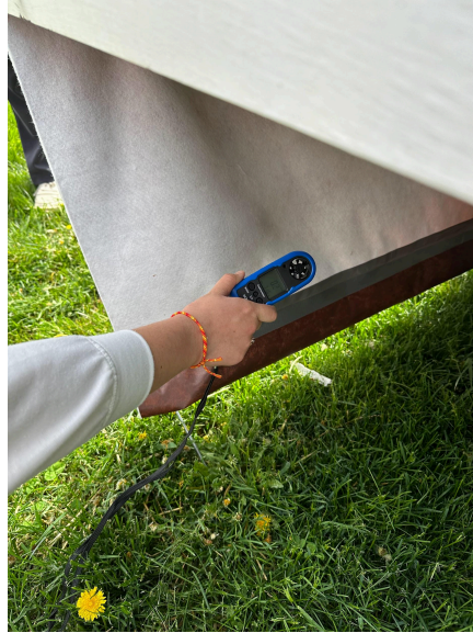
Fig. D5. Testing Fabric without wood or stakes with anemometer
