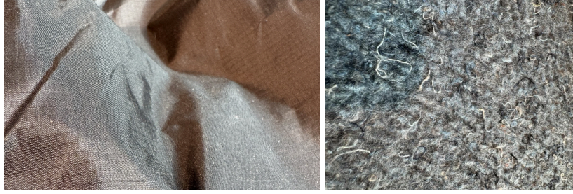
Fig. 6. Insulation and Ripstop Fabric Used for the Skirt
